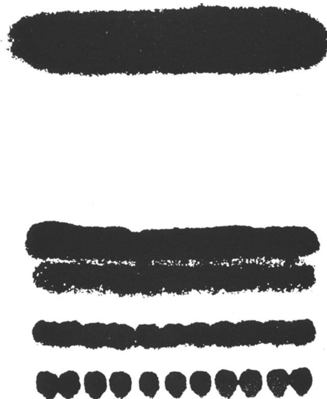
FIG. 1. Thin-layer chromatogram of a standard mixture of fatty acid methyl esters. The chromatogram was developed with 15% diethyl ether in hexane. The spots were located by charring after spraying with 50% sulfuric acid, and the reproduction was obtained by direct photocopy of the plate.
